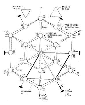
Figure 1 The rhombohedral arsenic structure projected onto  $(111)_{\rm rh}$ . The atoms (open circles) are labelled with the values of their parameters (numerically x = z for rhombohedral or hexagonal cells) referred to the origin (small square) in the centre; crosses (+) mark the lengths assigned to x and y in the Cartesian axial system.
